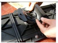
The O-ring gasket has to be put into the groove.
