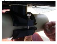
The two clamp saddle parts have to be connected to each other by screw, washer and self-locking nut (M8). The thread of the hexagon screw should be lubricated beforehand to avoid seizing.
